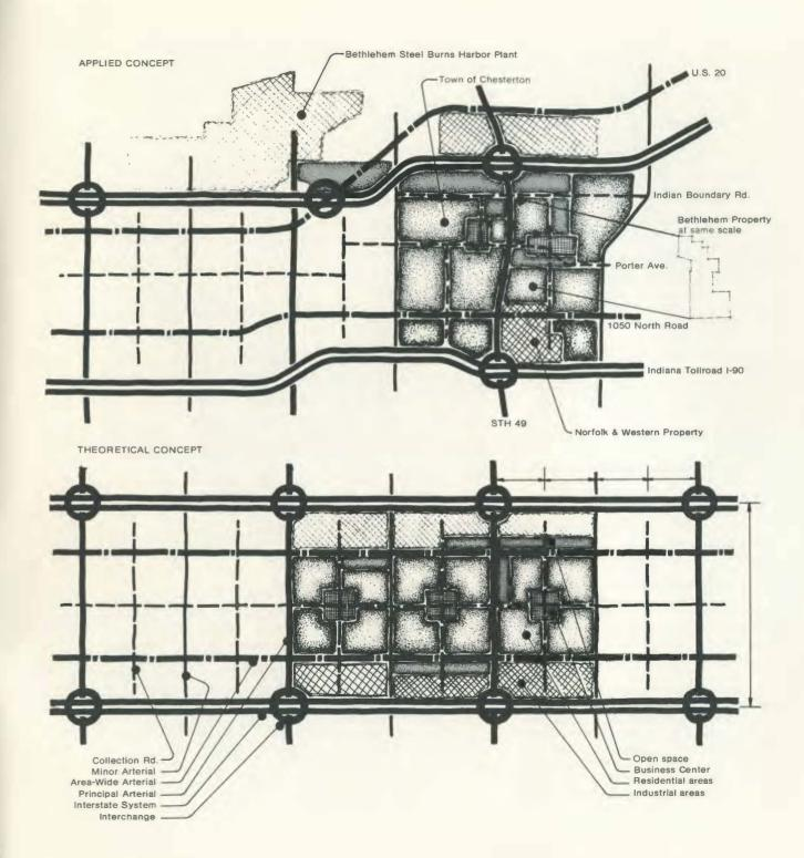
High-Accessibility Corridor Concept. This recommended concept is based on the principle of relating land uses and the level of accessibility they require to transportation systems and the level of accessibility they provide.
